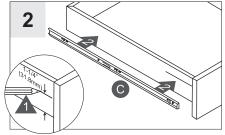
Mark 1-1/4" (32mm) from the bottom of the drawer side panel. Align the top of the drawer member (C) with
